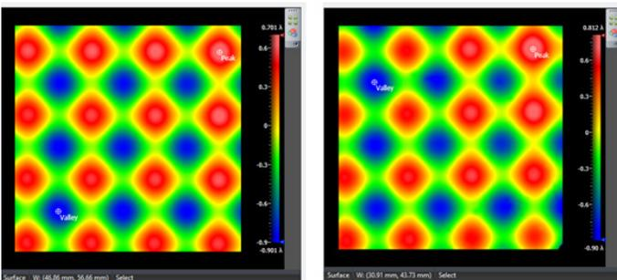
Replication from master to product for non-standard shapes can maintain high fidelity. In this example the Peak to Valley change from Master to Final Replica  $0.008 \text{ mm} \approx 0.8\%$
